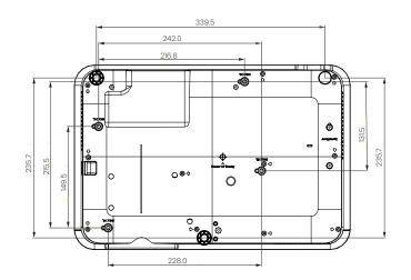
Ceiling/Wall mount screw: M4 (Max L = 25 mm; Min L = 20 mm) Unit: mm
